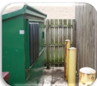
Keep the dumpster at least 3 feet from walls, fences and poles
